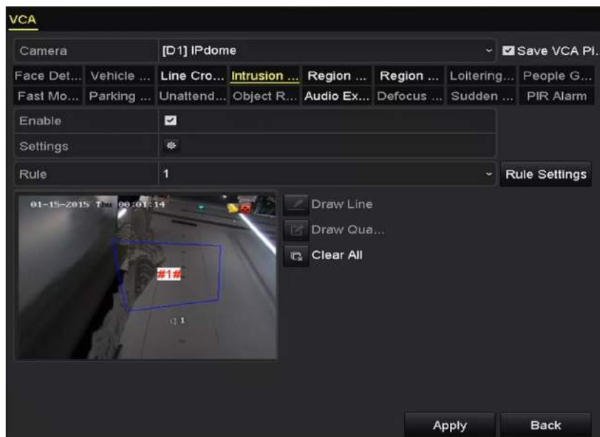
Figure 10-8 Draw Area for Intrusion Detection
